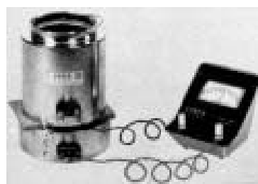
Fig. 2. Thermal Conductivity Apparatus, with constant temperature source above the slab and receiver, and with connections to the galvanometer.
