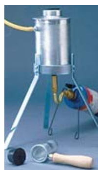
Fig. 5. The Steam Generator
