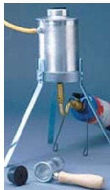
Fig. 7. The Steam Generator
