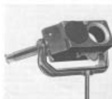
Fig. 6. The Lummer-Brodhun Photometer Box.
