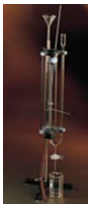
Fig. 3. Charles' Law Apparatus, or constant-volume air thermometer
