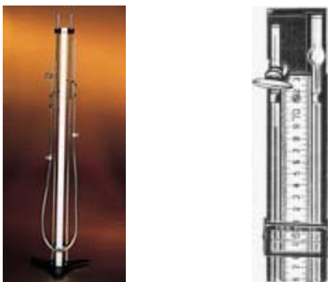
Fig. 5. Boyle's Law Apparatus. The insert shows a "close-up" of the upper end of the tubes.
