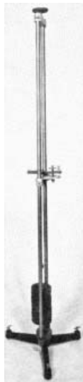
Fig. 5. Apparatus for determining Young's modulus. In this experiment the micrometer screw and level shown mounted on the bridge are replaced by the optical level shown in Fig. 4.
