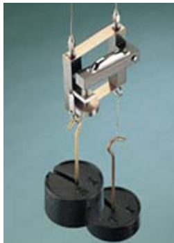
Fig. 2. Apparatus for determining Young's modulus using a scale and vernier.
