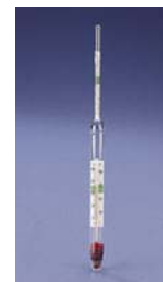
Fig. 6. Hydrometer for measuring specific gravities of light liquids.
