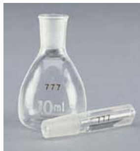
Fig. 1. Specific Gravity Bottle for determining densities of liquids.
