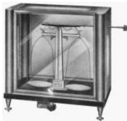
Fig. 2. Balance for determining masses of specific gravity bottles.
