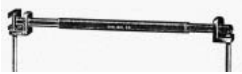
Fig. 8. Apparatus for diffraction measurements with light shield. For use in undarkened room.
