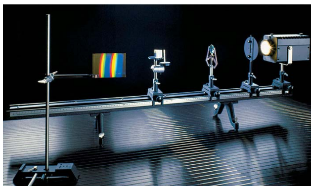
Fig. 6. Lathe bed form of optical bench.
