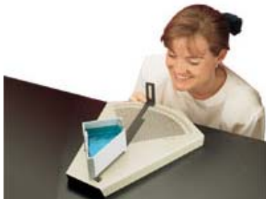
Fig. 4. The Refraction Apparatus. When the tank is partially filled with a transparent liquid, one can see the slit that hangs on the back plate of glass by sighting either through the liquid or above it. By using the index arm, one can measure the angle of refraction and the corresponding angle of incidence of light traveling from water into air.
