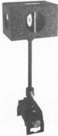
Fig.5 Bunsen photometer (complete)
