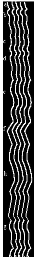
Fig. 4. Typical traces made by a falling fork.
