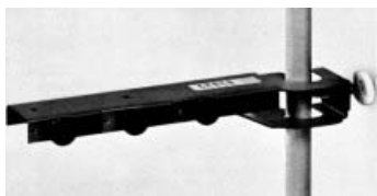
Fig. 3. Suitable clamp for supporting a simple pendulum.
