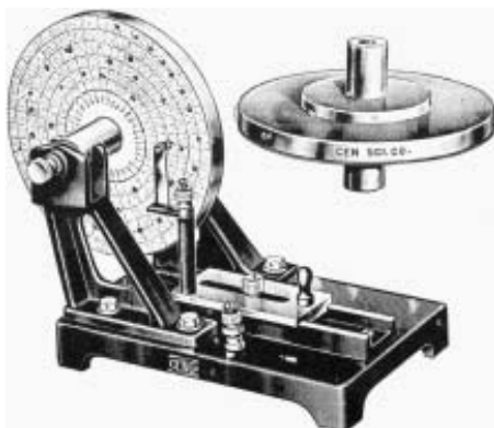
Fig. 3. Rotational Inertia Apparatus. The insert shows the three-step disk. The wheel is shown covered with the coated-paper chart with polar-coordinate rulings.
