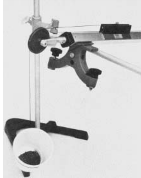
Fig. 4. Operational setup for the inclined-plane experiments.
