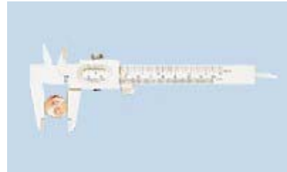
Fig. 5. A metric-scale vernier caliper.
