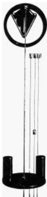
Fig. 4. Torsion Pendulum with disk, cylindrical masses, ring and various rods.
