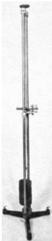
Fig. 4. Apparatus for determining the torsion constant of a wire and the rotational inertia of a ring. The ring and disk are shown mounted on the apparatus which is conventionally used for the determination of Young's modulus.
