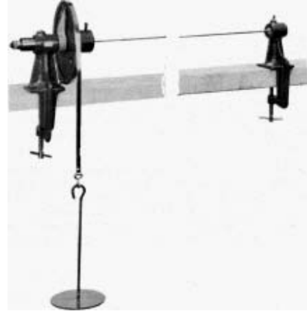
Fig. 3. Apparatus for determining the modulus of rigidity of a substance in the form of a cylindrical rod.
