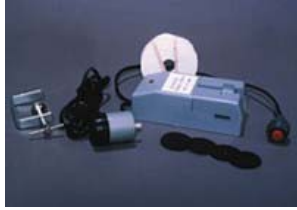
Fig. 6. Spark Timer, producing sparks at intervals of 1/60 second.
