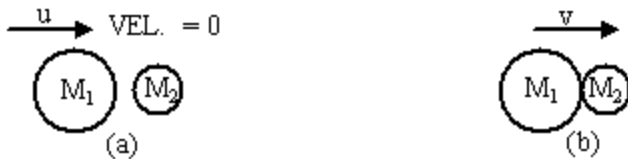
Fig. 1. Inelastic collision of two objects: (a) Velocities before impact; (b) Velocity after impact.
