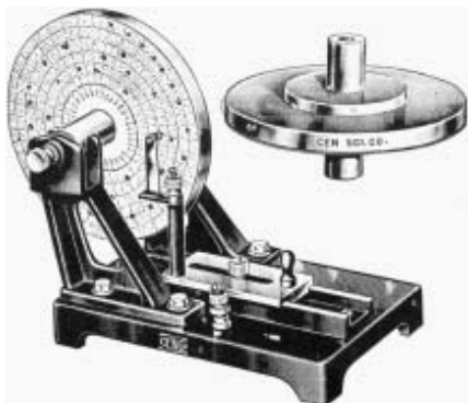
Fig. 3. Rotational Inertia Apparatus. The wheel is shown covered with the coated-paper chart with polar-coordinate rulings.
