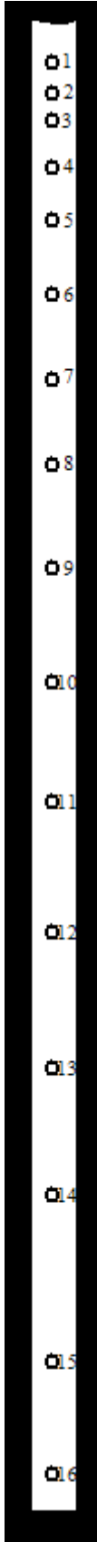
Fig. 8. Spark record of the freely falling body of the Free Fall Apparatus. The illustration is one-sixth actual-size.
