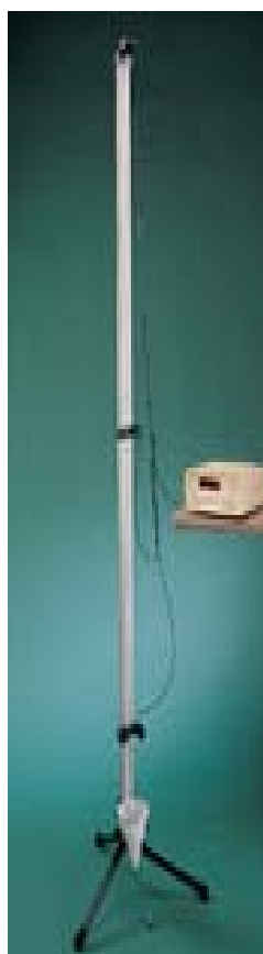
Fig. 1. Free Fall Apparatus. Electrical connections can be conveniently made from the accessory apparatus, when arranged on a nearby table.
